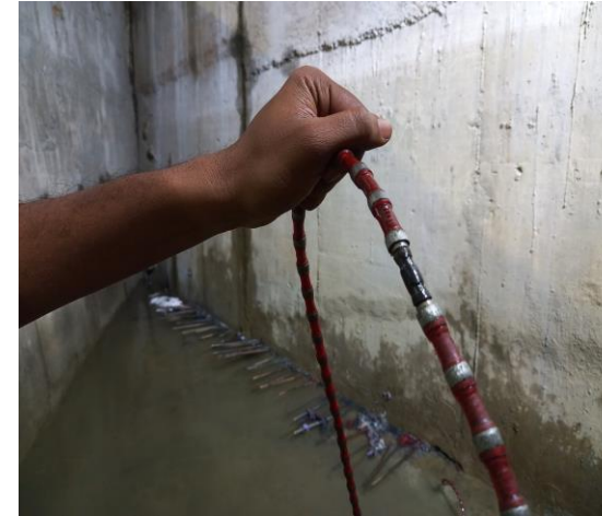
More than 70mts of diamond wire rope.
