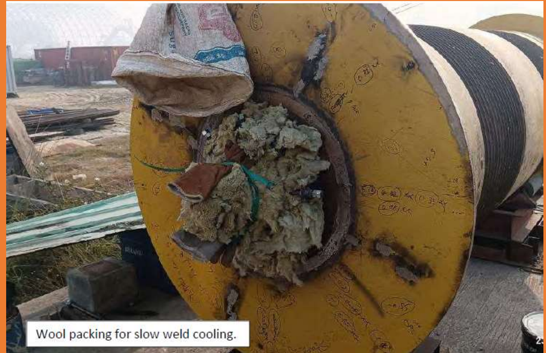
11. Slow cooling done by glass wool packing.
