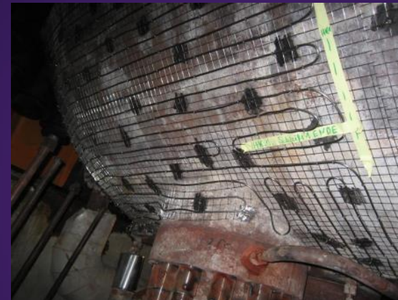
Electric heating coils to keep HP/ IP Turbine casing and shaft in warm start conditions
