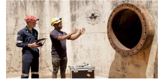
Spherical cage mounted drone
