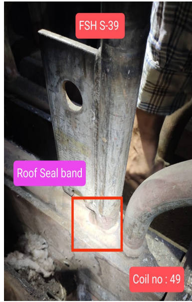
Seepages observed in Shop welded attachment lifting lug joints & Roof Seal band area in Finish Superheat (FSH) inlet Super 304H coils (S-39) of during 1 st Hydrotest
