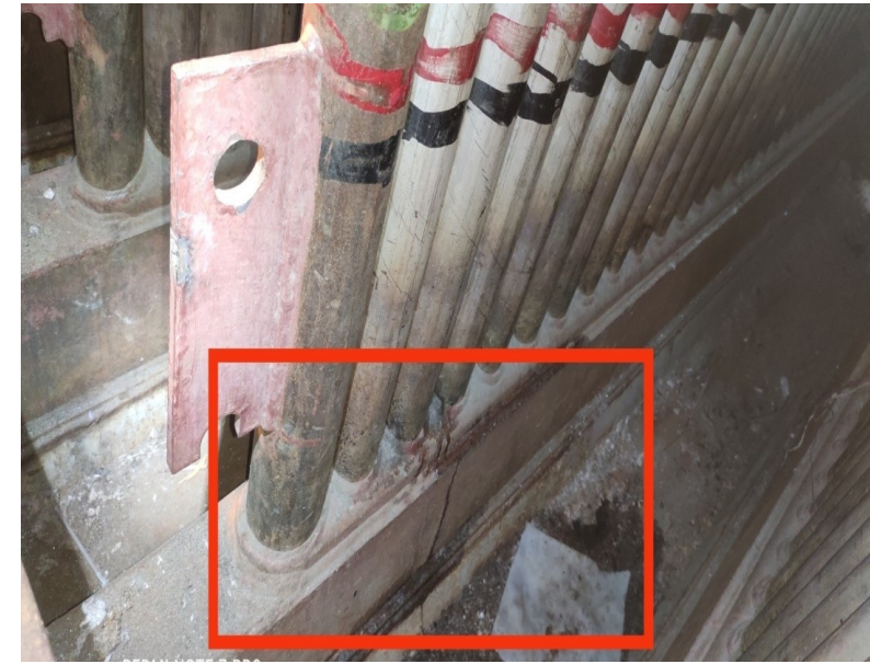
Observed seepages in 29 tubes near SHOP WELDED Seal band joints of Finish Reheater (FRH) coils during 1 st hydrotest
