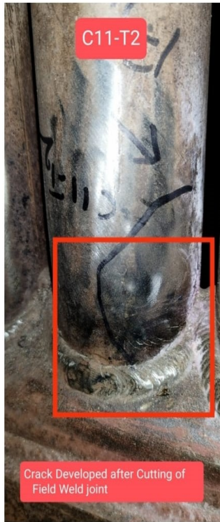
FRH coil tubes near Seal band weld lost it's ductility!
