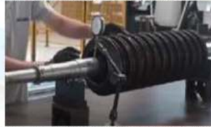
(Figure 2. Runout Inspection at Flat Surface of Vadodara RES.)
