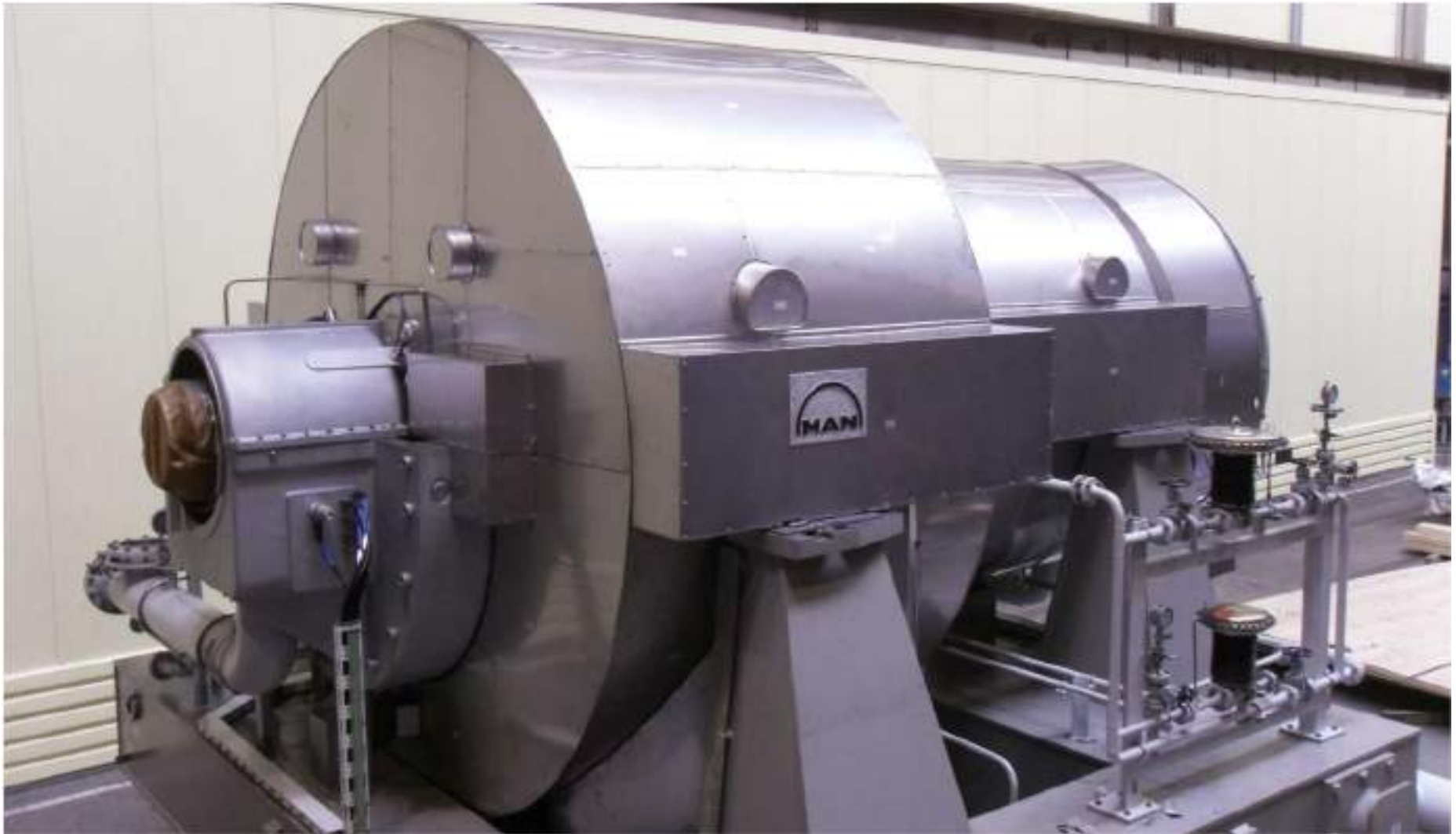
Metal jacketed noise insulation of compressor
