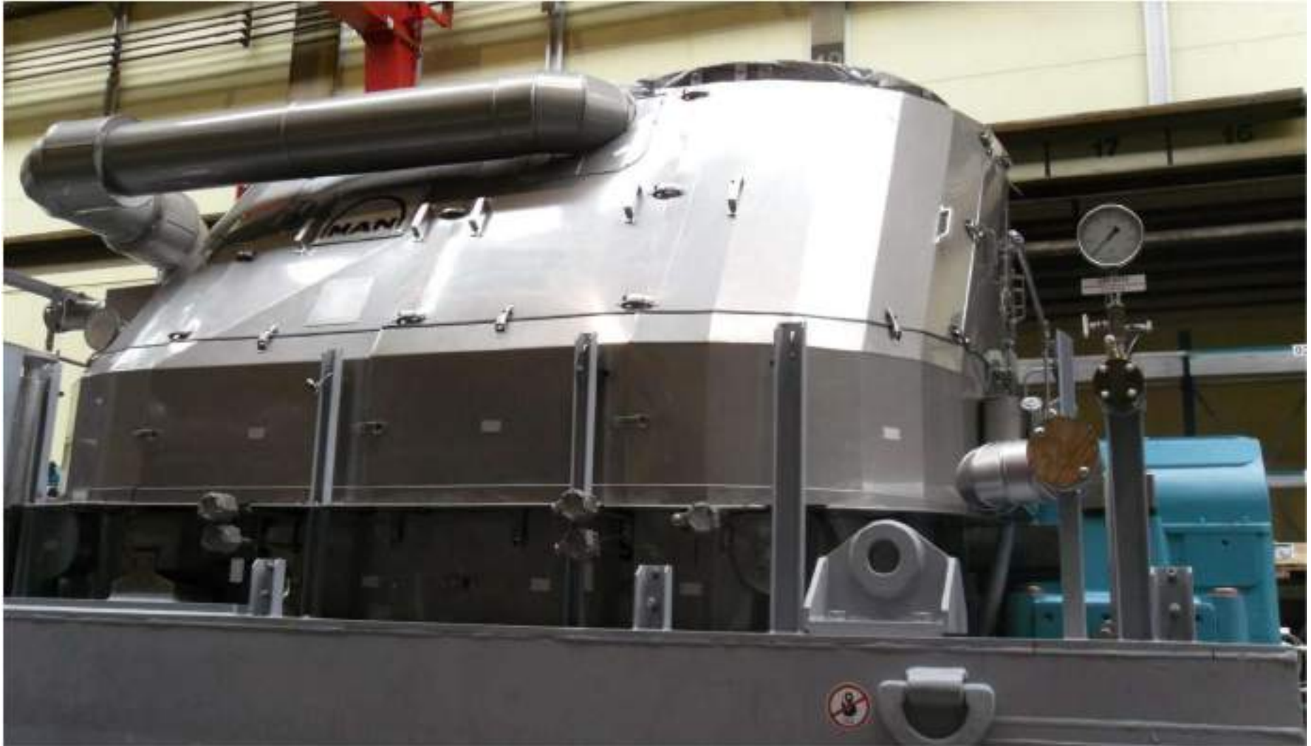
Fast and tool free assembled cassettes insulation system for heat and noise reduction of gas expander
