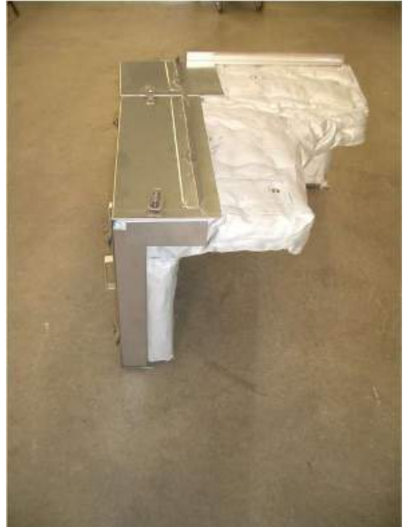
Turbine joint insulation cassette
