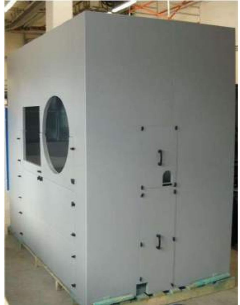
Noise insulation on industrial gear
