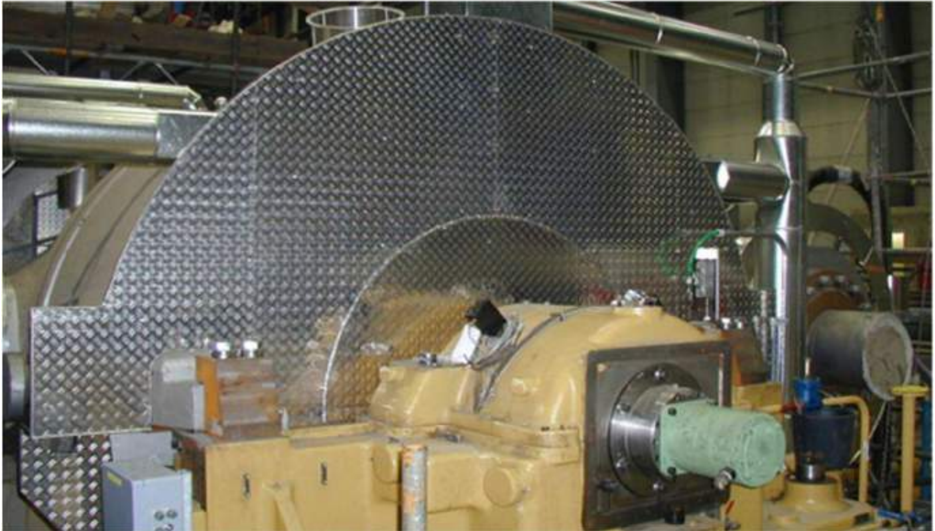
Heat retention shield made of duet stainless steel sheet
