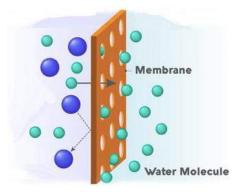
Filter water through the membrane filter wall and produces clean water
