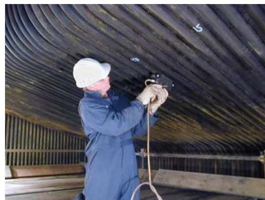
OD Scanning of Water Wall Tubes at various sections of the Boiler
