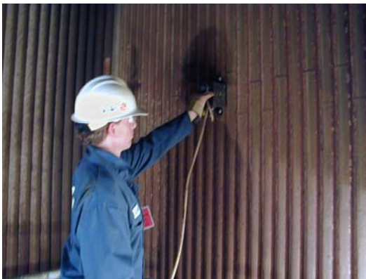
OD Scanning of Water Wall Tubes at various sections of the Boiler
